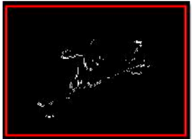
Figure 2: Binary Image interpreting the bit value of 0 as black and 1 as white
